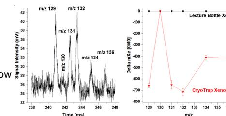
Figure 11: Cryotrap column xenon spectra averaged over 250 scans and 3 trials.
