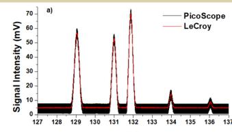
Figure 7: Xenon spectra at fixed x-axis (5 MSa/s) and y-axis (8-bit) resolutions
