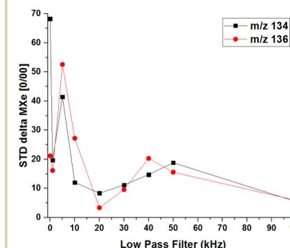
Figure 10: Standard deviation with respect to m/z 134 and 136 at varied LPF settings for m/z 134 and 136
