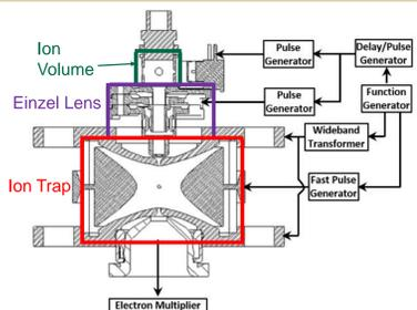
Figure 1: Electronics configuration for ion trap
