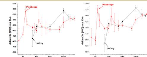
Figure 8: Sampling rate (x-axis) study on xenon isotopes m/z 134 and 136 for each DAQ system
