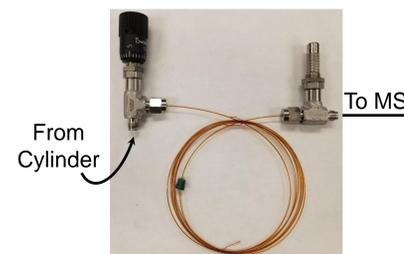
Figure 5: Trapping column coupled to ion trap
