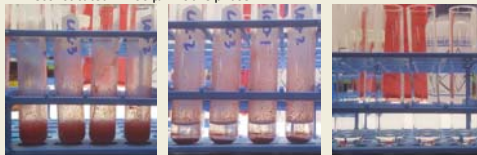
Figure 4 – After vortex Figure 5 – After centrifuge Figure 6 – After decant
