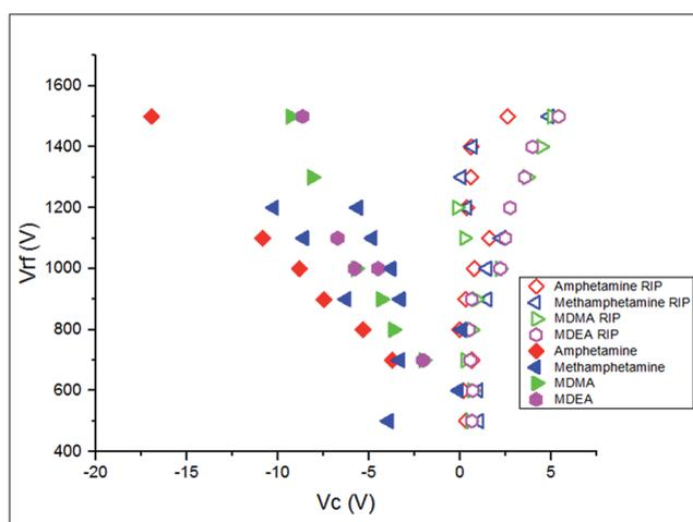
Fig. 5 Dispersion tracks of neat drug samples following dispersed and residual ion peaks (no reaction chamber employed).
