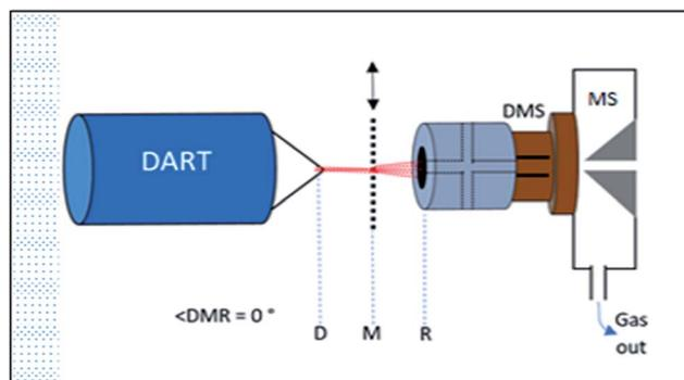
Fig. 3 Schematics of DART-DMS-MS setup. Sample is deposited on a mesh screen (M) mounted on a motion stage moving orthogonally to the direction of ions. The angle between the DART source (D), mesh screen (M), and reaction chamber inlet (R) is at  $0^\circ$ . Where  $|\text{DM}| = 6 \text{ mm}$  and  $|\text{MR}| = 6 \text{ mm}$ . The reaction chamber was designed to accommodate the supply of dry nitrogen gas and isopropyl alcohol vapor to improve DMS separation.
