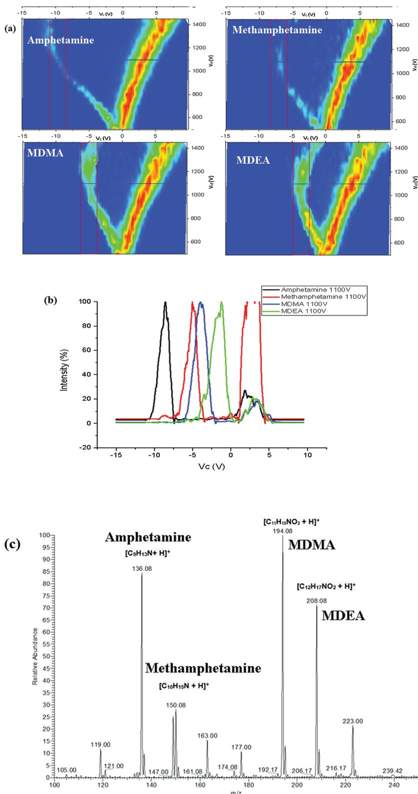
Fig. 7 (a) Dispersion plot of the extracted ion masses of amphetamine, methamphetamine, MDMA and MDEA ions as they are separated from the RIP. (b) At a fixed  $V_{rf}$  of 1100 V, the ions were transmitted at  $V_c$   $-9.0$  V,  $-5.0$  V,  $-4.0$  V and  $-2.5$  V respectively. (c) Mass spectrum of protonated amphetamine, methamphetamine, MDMA and MDEA of  $m/z$  136, 150, 194 and 208 respectively at all  $V_c$ .
