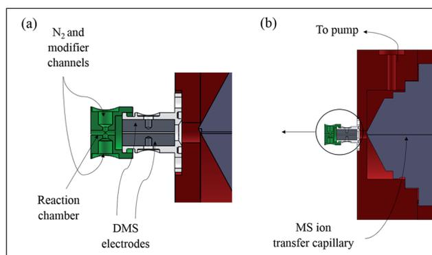
Fig. 4 DMS-MS set-up. (a) Detailed view; and (b) full view.
