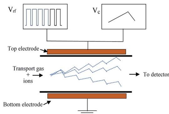
Fig. 1 Concept of differential mobility spectrometry.
