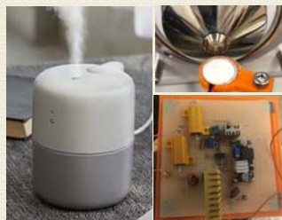
Figure 2. Home-built ultrasonic nebulizer ionization source.
