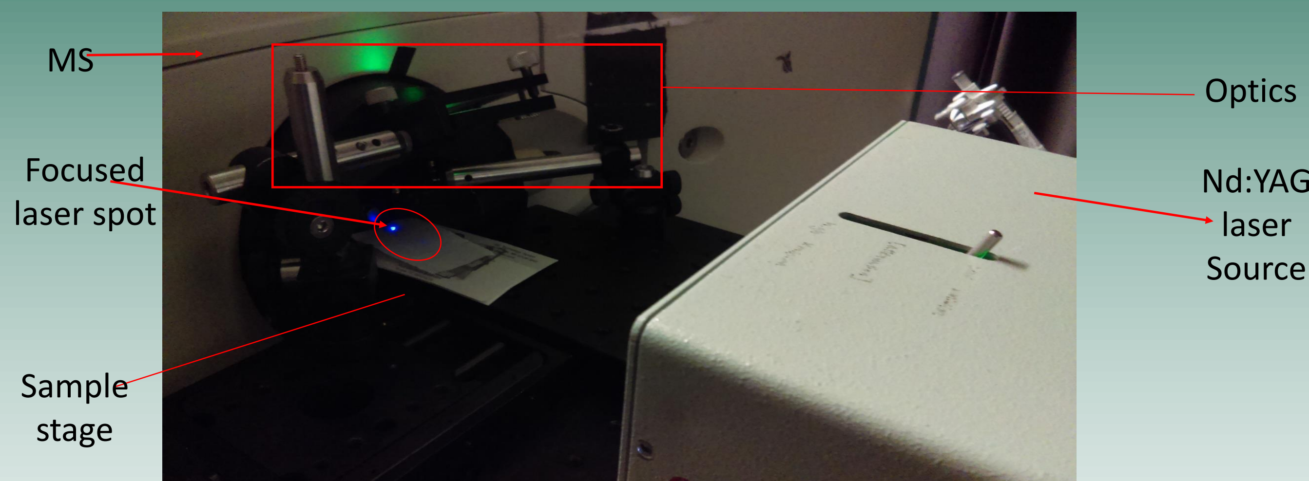
Figure 4. Laser desorption ionization mounted to interface with the MS inlet
